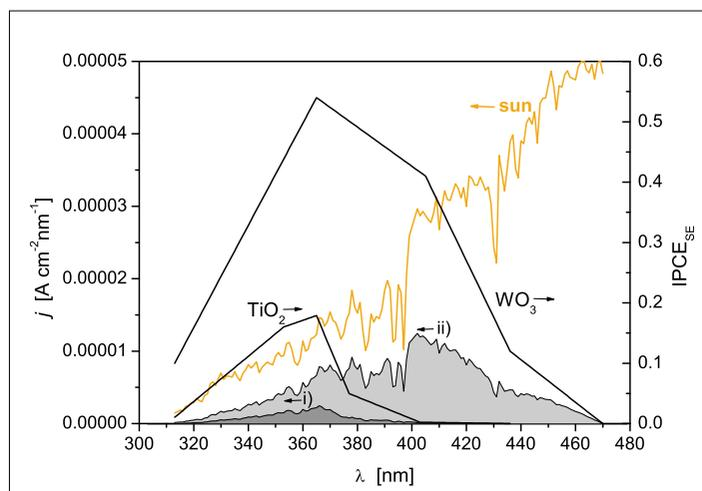
Fig. 3. Comparison of the total photocurrent that can be obtained from semiconductors of different bandgap. Curve i) ...  $j \cdot \text{IPCE}_{\text{SE}}(\text{TiO}_2)$ , curve ii) ...  $j \cdot \text{IPCE}_{\text{SE}}(\text{WO}_3)$ . The light intensity,  $j$ , of sunlight is expressed as current density.
