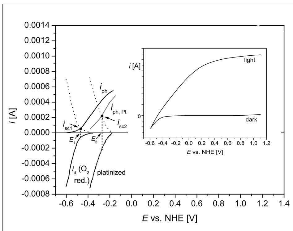
Fig. 1. Influence of dark currents (oxygen reduction) on local cell currents ( $i_{sc}$ ) on an illuminated TiO<sub>2</sub> electrode (photocurrent onset region). The electrolyte (0.1 N NaOH) was saturated with oxygen and stirred; scan rate:  $-0.5 \text{ mV/s}$ , ( $i_d \dots$  dark currents for O<sub>2</sub> reduction, photocurrent ...  $i_{ph} = i_{\text{light}} - i_{\text{dark}}$ ). Inset: current - potential curves under light and in the dark over a wide range of potentials.
