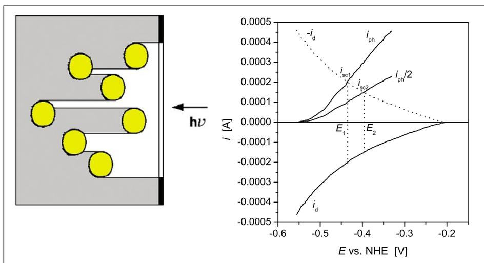
Fig. 4. Sharing of a given number of photons by several particles suspended in solution. Left: illumination of a particle suspension through a mask (schematic), right:  $i$ - $E$  curves for light being absorbed by one or two particles.  $i_{ph} = i_{light} - i_d$ .
