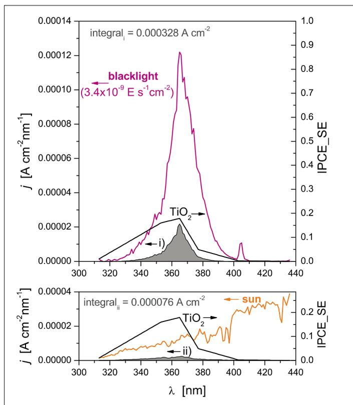
Fig. 2. Influence of light source on the total photocurrent that can be obtained under depletion conditions. Upper part: curve i) ...  $j \cdot \text{IPCE}_{\text{SE}}(\text{TiO}_2)$  with the light intensity,  $j$ , of the blacklight source expressed as current density, lower part: curve ii) ...  $j \cdot \text{IPCE}_{\text{SE}}$  with the light intensity,  $j$ , of sunlight expressed as current density.
