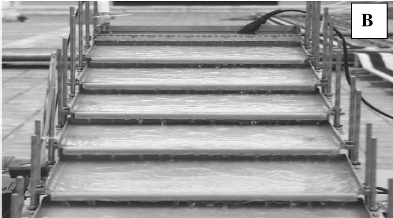
**Figure 3. Waste water treatment by solar energy using tubular (A) and flat sheet (B) reactors**
